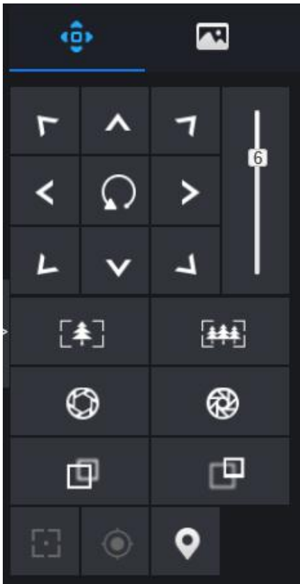
Figure 8-11 PTZ control interface
