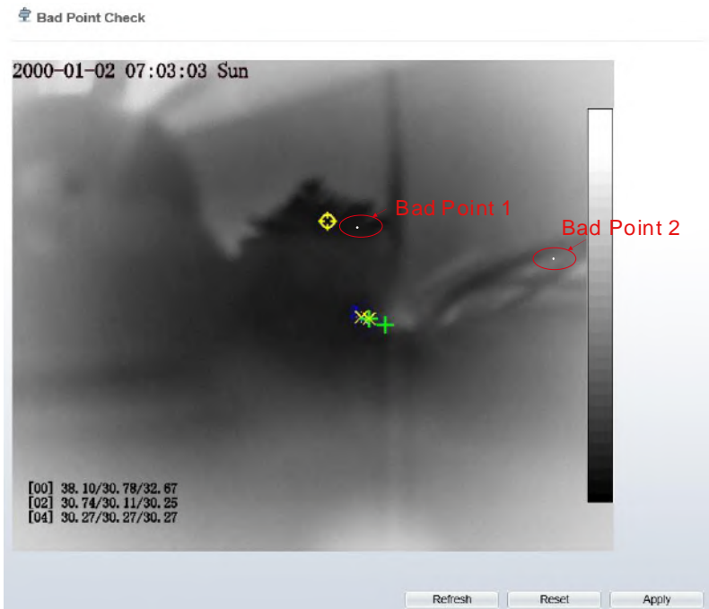
Figure 4-15 Bad Point Check
