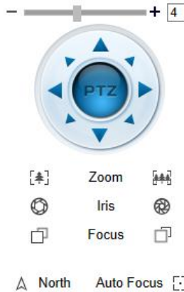
Figure 7-1 PTZ Control zone
